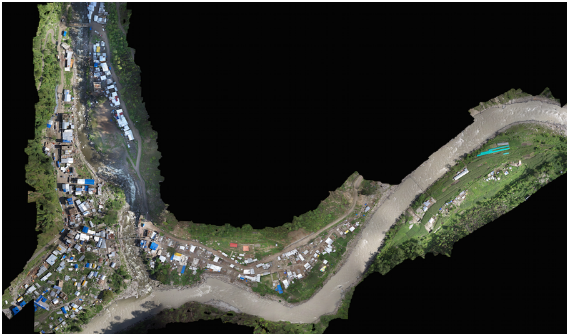
Fig. 2 Orthophotograph prepared by 869 photographs taken by a drone in Shingati.
